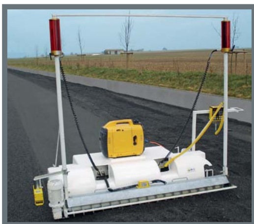
» Minigrader used in the construction of a bikeway – equipped with a MOBA Dual-Laser-matic
